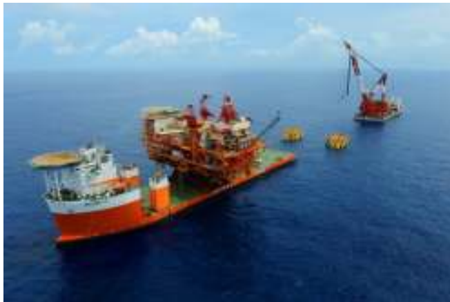
Float-Over Standoff Phase. HZ25-8 DP-South China Sea
