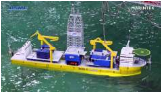
Control System Model Test
