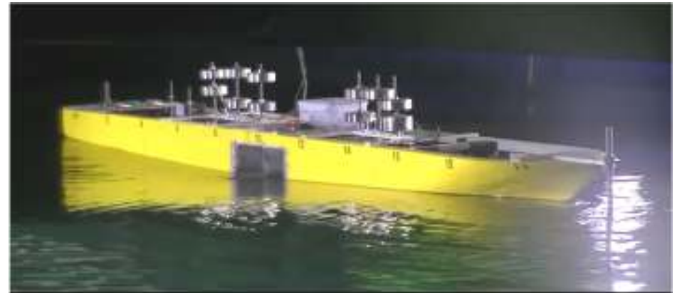
Damaged Condition \lambda/H = 1.0
